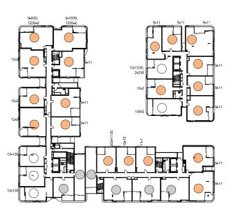
03 TYPICAL LEVEL 02-03 - SCALE: 1:500@A1 SOLAR ACCESS: 20/31 NO SOLAR ACCESS: 6/30
