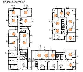
04 TYPICAL LEVEL 04-05 SCALE: 1:500@A1 SOLAR ACCESS: 21/31 NO SOLAR ACCESS: 6/31
